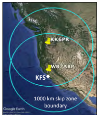
Fig. 1. Map showing transmitter and receiver locations. Circles show a 1000 km skip zone.
